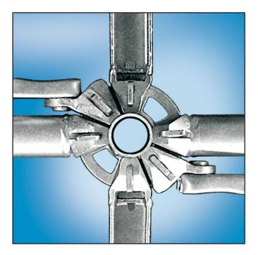
Developed for one-man assembly, irrespective of height, scaffolds can be constructed in three dimensions from each rosette. Ledgers or transoms are connected at right angles with additional components then added at a choice of angles. Installations are automatically centred and correctly located for safe assembly.
